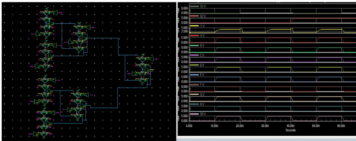
Fig 4.2: CMOS 8X1 mux Schematic design and output wave form
