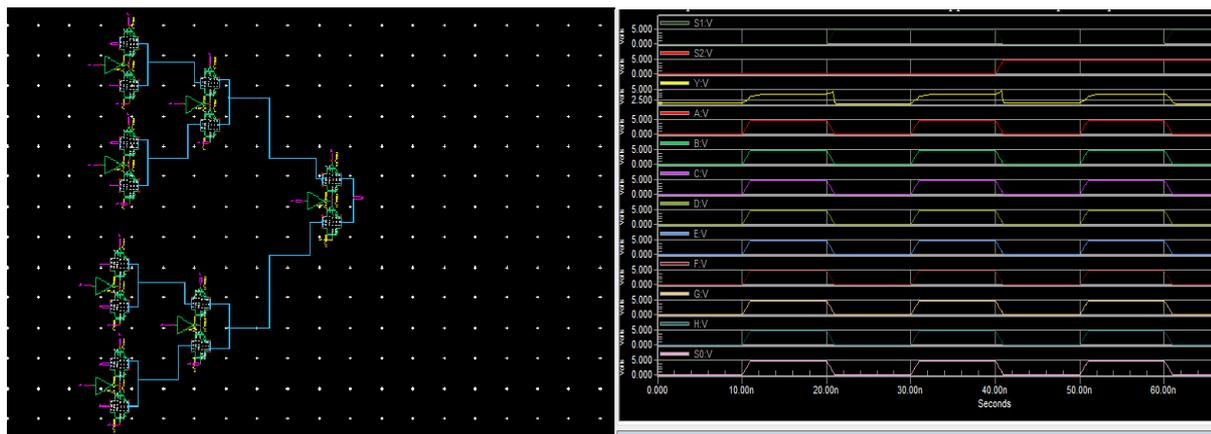
Fig 4.4: TG 8X1 mux using Schematic design and output wave form
